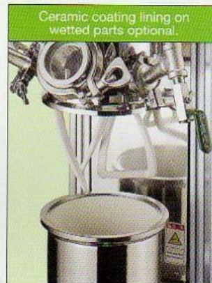
▲ Photo: Model 2P-1 Vessel with half-jacket is optional.
